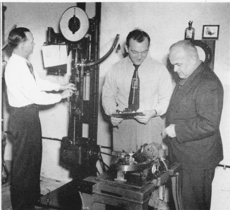
the zipper sideways until it pulls apart, registers the number of pounds it takes to break a zipper.
